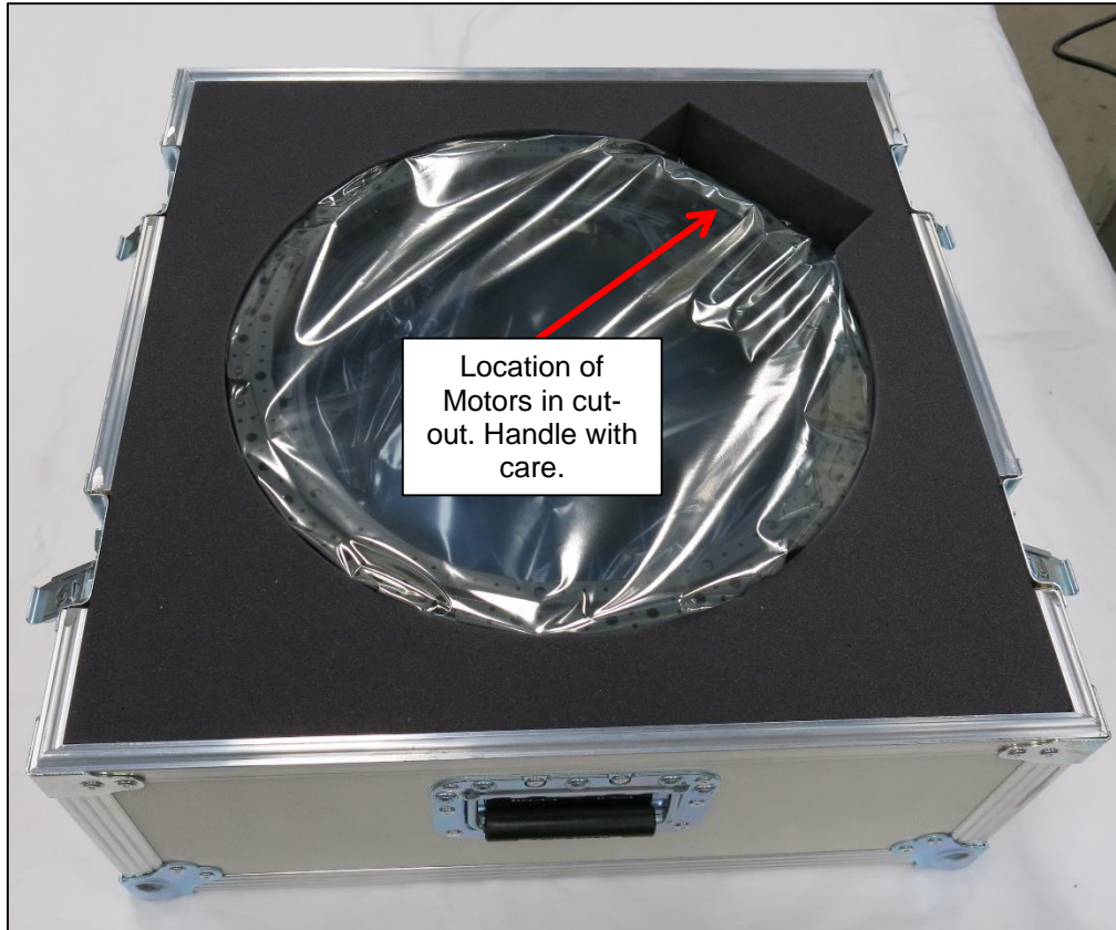
Figure 3-4: Lightband with Motor Bracket aligned to cut-out inside the shipping container foam
