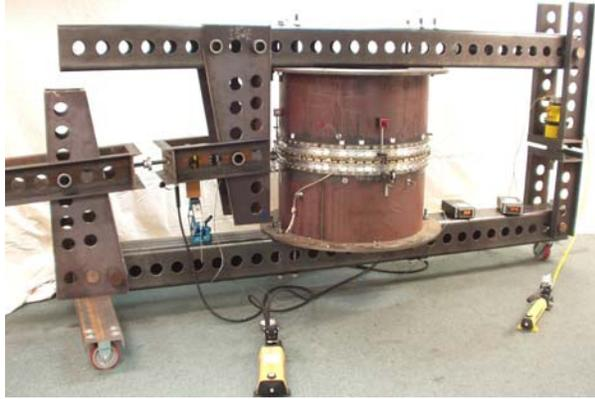
**Figure 12 Strength test fixture**
