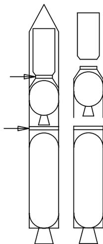
**Figure 1 Launch and space vehicles need separation systems**
