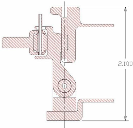
**Figure 10 Cross-section of Motorized Lightband. Dimensions are in inches.**
