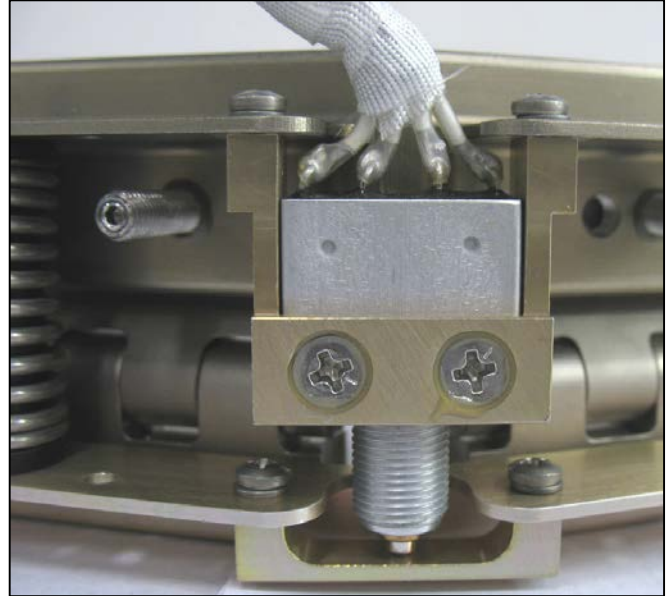
Figure 16: Lower switch bracket installed on upper ring. Upper switch bracket installed on lower ring. Harness is taped and formed.
