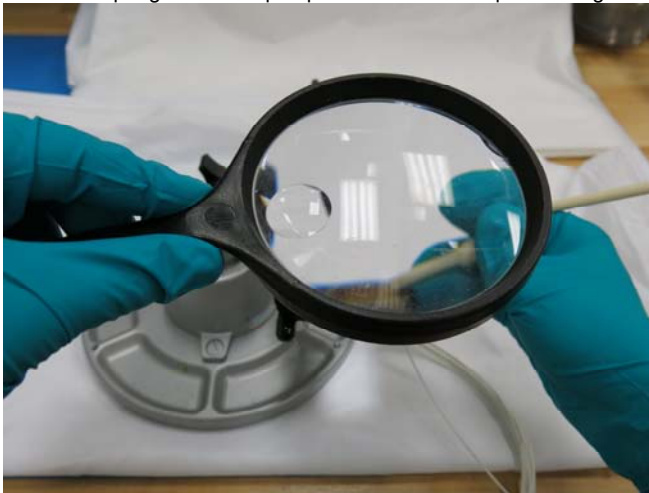
Figure 27: Use clean blunt edged plastic pick to compress spring contacts
