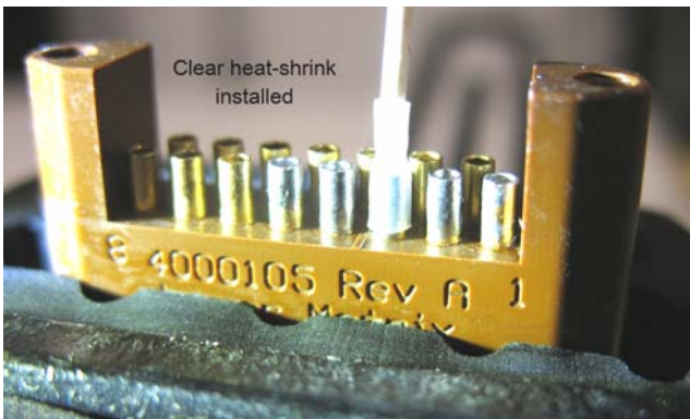
Figure 12: Heat shrink installed
