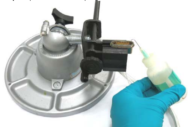
Figure 24: Squirting the spring contacts with IPA
