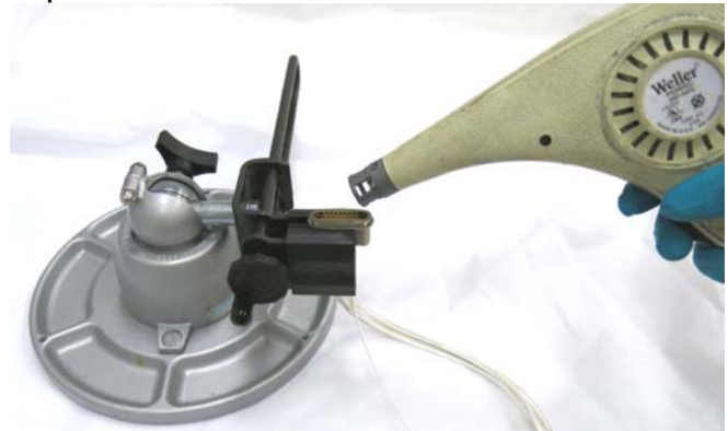
Figure 29: Heating the connector back shell to evaporate any remaining IPA
