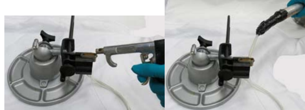
Figure 28: Spraying with clean compressed air and vacuuming connector
