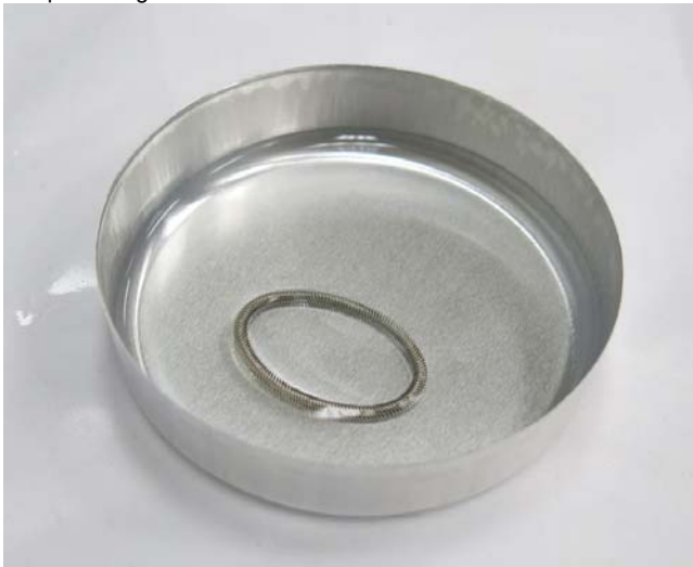
Figure 22: EMI gasket in clean IPA bath
