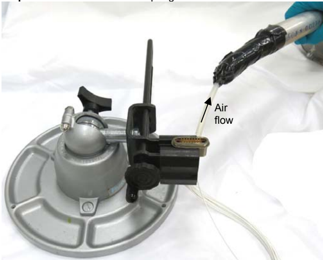
Figure 26: Vacuuming connector spring contacts with custom vacuum attachment
